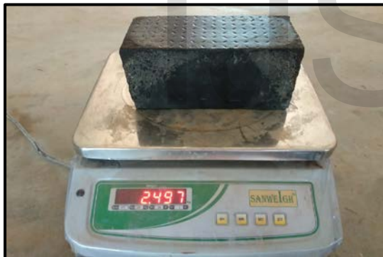
Figure 10: Weighing of Plastic Soil Brick
