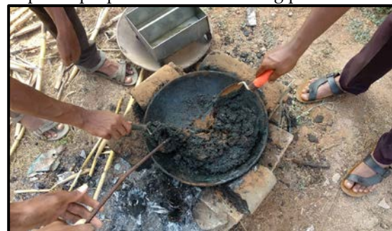
Figure 6: Mixing of molten plastic and graded soil
