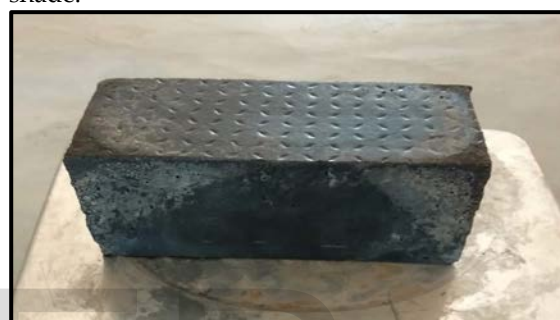
Figure 13: After efflorescence test on Plastic Soil Brick
