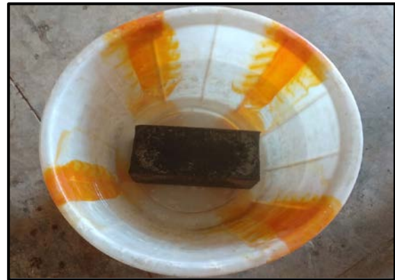
Figure 11: Water absorption test on Plastic Soil Brick
