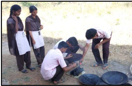
Figure 7: Moulding and compacting the mix of plastic and soil
