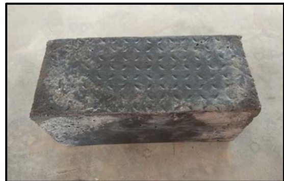
Figure 9: Plastic Soil Brick
