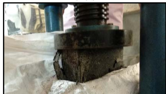
Figure 12(a): Compressive test on Plastic Soil Brick
