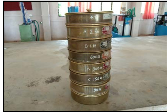
Figure 1: Sieves used to sieve the soil
