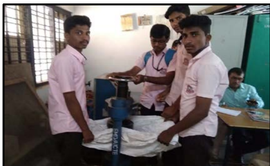
Figure 12(b): Compressive test on Plastic Soil Brick
