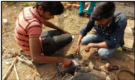
Figure 8: Giving Finishing to the brick surface
